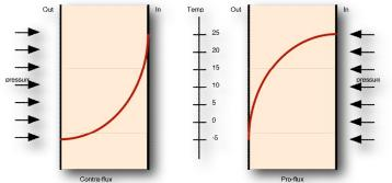
Because the air is always moving to the warm side, where its potential to hold moisture increases, and because at typical ventilation rates the velocity of the incoming air overcomes the outward diffusion of water vapour, condensation cannot occur. Provided that the air continues to flow then the building membrane effectively creates its own vapour barrier.
