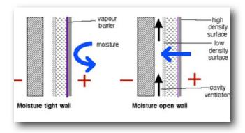
Since the 1980's there has been a development of designed naturally ventilated and moisture transfusive buildings. The moisture transfusive wall encourages moisture flow outward into a ventilated cavity and dispenses with a vapour barrier. It reduces build up of moisture resulting from activities inside a space.
